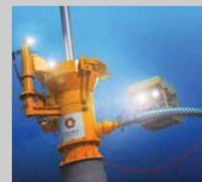
Riserless Mud Recovery (RMR®) is a risk-reduction system that allows you to drill a better, more stable top hole safely, quickly and with less environmental impact.
