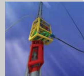
EC-Drill® is a Managed Pressure Drilling (MPD) system based on a Dual Gradient Drilling (DGD) method. It can be used in both shallow and deep water (including depleted wells), either from a jack-up, platform or a floating drilling vessel.
